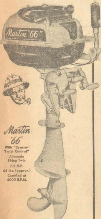
The new MARTIN "66" combines the power and stamina of the famed MARTIN 7.2 H.P. motor with the "Synco-Twist Control" for new operating ease... speed, spark and steering are controlled while you face forward.
